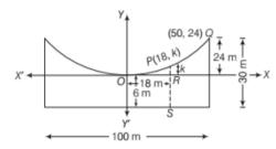
Focus is at the middle of the cable and shortest and longest vertical supports are 6 m and 30 m and roadway in 100 m long.
